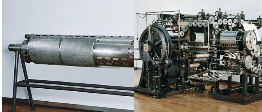
**Plate cylinder of a rotary
