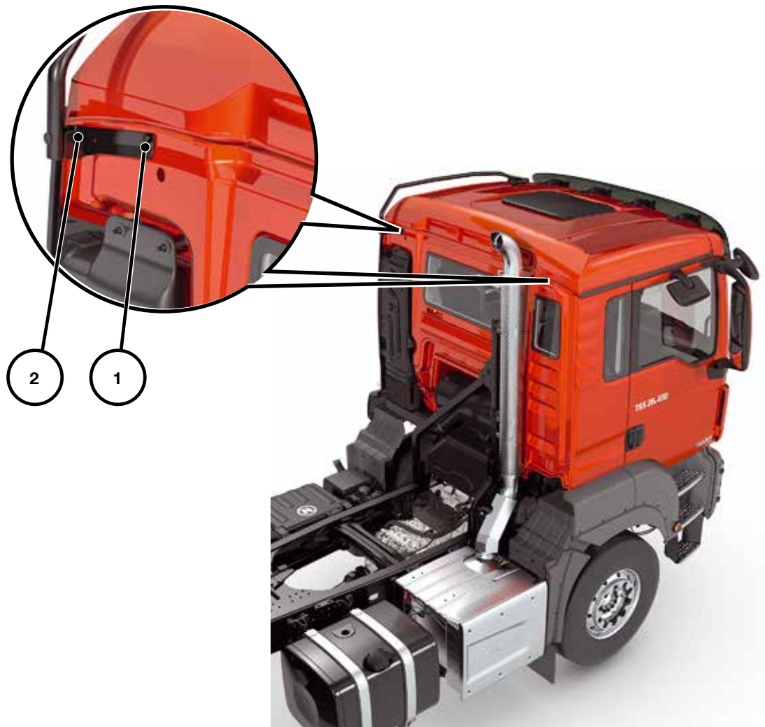
Fig. 29-III: Additional fastener for roofwalk
