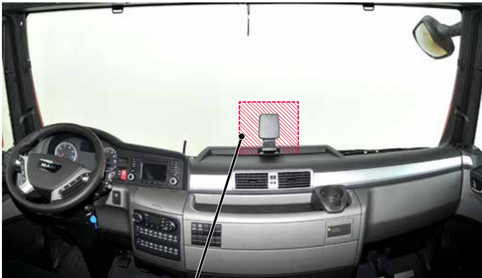
Fig. 144-III: Cab interior with multi-functional camera
