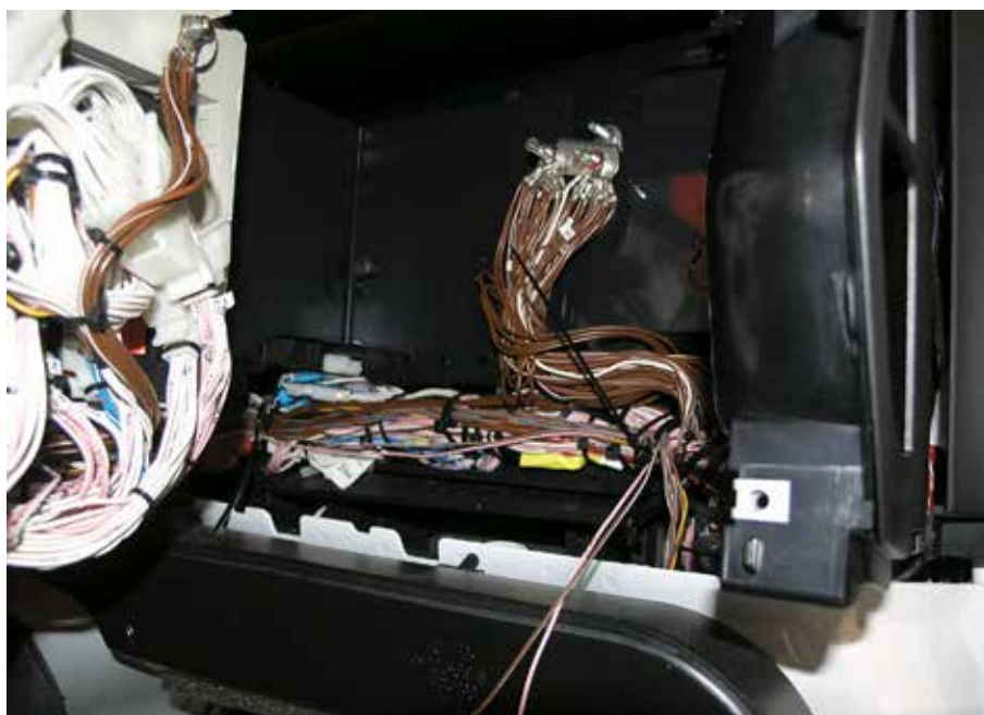
Fig. 137-III: Ground point X1644 behind central electric unit
