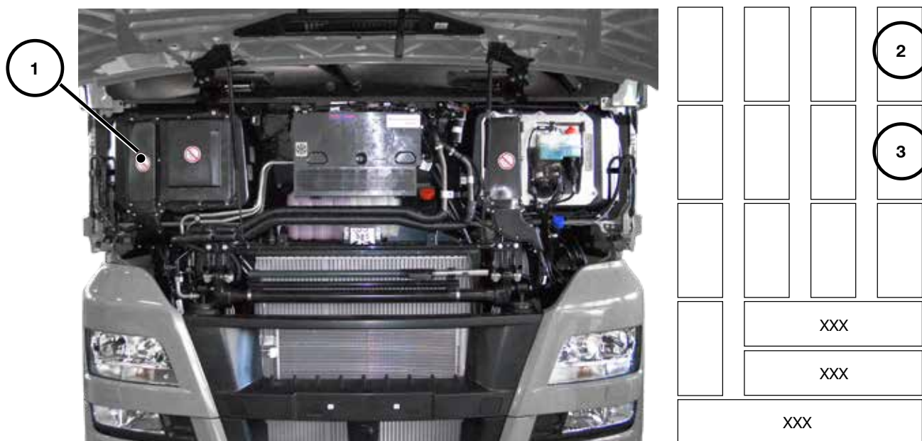
Fig. 128-III: Installation location of ISC interfaces
